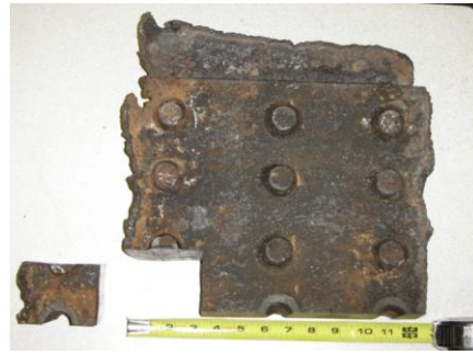
Plate A-6 with Rivet Portion Removed
